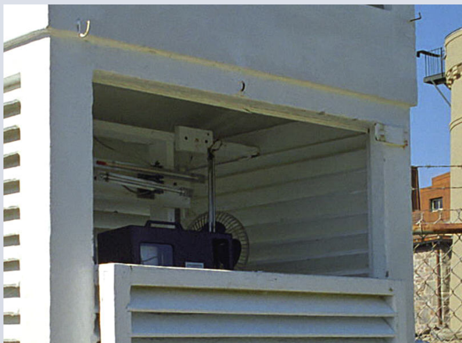
Hazen instrument shelter at Blue Hill with hygro-thermograph and thermometers.
